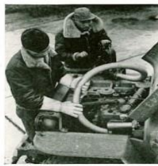
Fig. 2. Using the 796-A Heater with accessory duct to heat the intake manifold of a Jeep.
