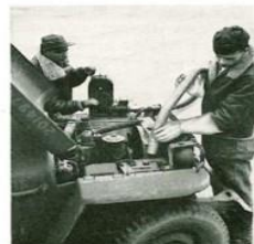
Fig. 3. Using the 796-A Heater with accessory duct to heat the battery of a Jeep.
